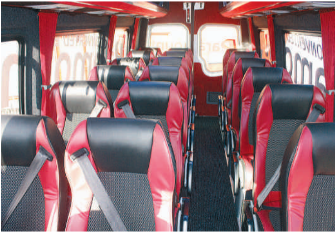
The 518's interior is luxuriously trimmed with 18 Politecnica Rally seats and full length rack systems incorporating individual passenger control panels.
