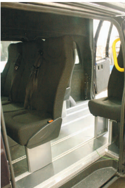
A wheelchair accessible Mercedes-Benz Vito under construction. It will have five passenger seats and an in-board lift.
