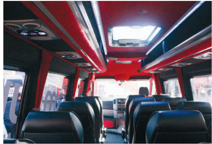
The 518's interior is luxuriously trimmed with 18 Politecnica Rally seats and full length rack systems incorporating individual passenger control panels.
